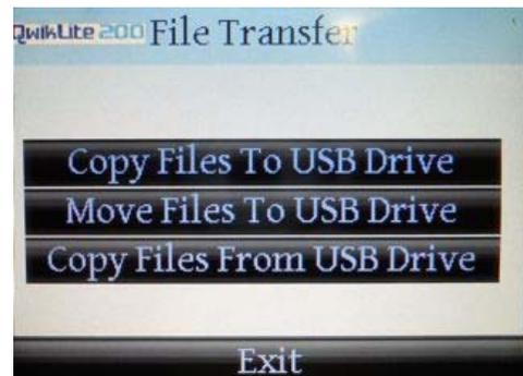
The "Copy Files To USB Drive" command will maintain a copy of all files on the QwikLite instrument.
