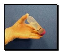
7. While the homogenous mixture remains in suspension, pipette 2 mL of solution from the conical mixing tube in to 3 cuvettes of the first CONTROL cartridge. Cap the conical tube and repeat the swirl procedure from Step 6 before pipetting the final 3 cuvettes. This ensures that culture will not settle to the bottom of the conical tube during Dosing. Pipette from the same point in the conical tube for every cuvette.
